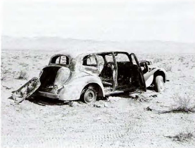
Buick four-door sedan placed at one-half mile from ground zero, with windshield oriented toward the blast. All windows were blown out, as was the rear of the car. The doors away from the blast were blown off their hinges, and the hood was blown some 50 to 100 yards from the car. Burning of the automobile was extensive. The rear tires were burned, and the car sank into the ground to the axle level. The front tires were undamaged and still inflated. The motor appeared to be undamaged. Source: Los Alamos National Laboratory.
